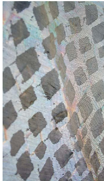
Printing with caustic soda and heat setting
